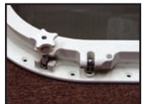
Hinge bolt and deadlight attachment detail
