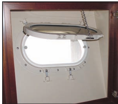
Oval portlight, Open with screen, Installed
