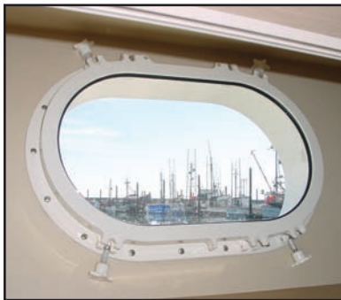
Oval portlight, Installed
