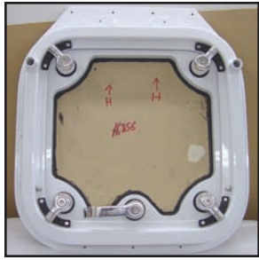
Deep gutter, Underside, Dogged
