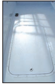
Installed in fiberglass Sport deck, Hinged short side, Closed
