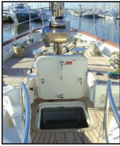
Surface hinges, Lever handle, Forepeak access, Open
