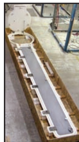
Two panel, Deck crane hatch
