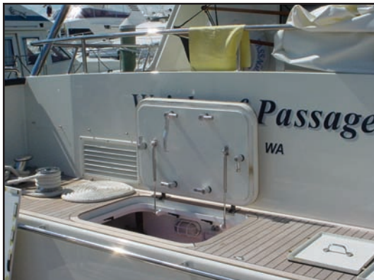
Shown in the open position, polished hardware and gas springs make this hatch an attractive addition to the aft cockpit.
