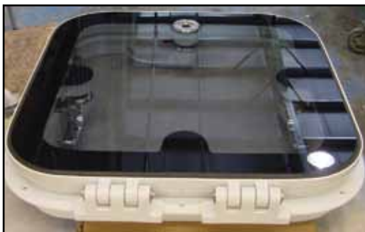
Below, Lens hatches, Proud / raised
