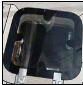
Installed flush with teak, Surface hinges, Interior handles only
