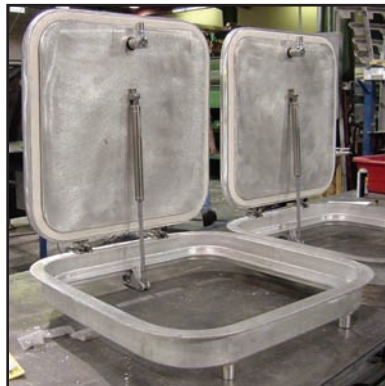
Single dog, Single gas spring, Surface hinges
