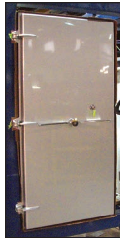
Custom watertight bulkhead door, Mitered corners, Finished to yacht standards, Lock (keyed outside, thumbturn inside), Custom stainless handle (Exterior view)
